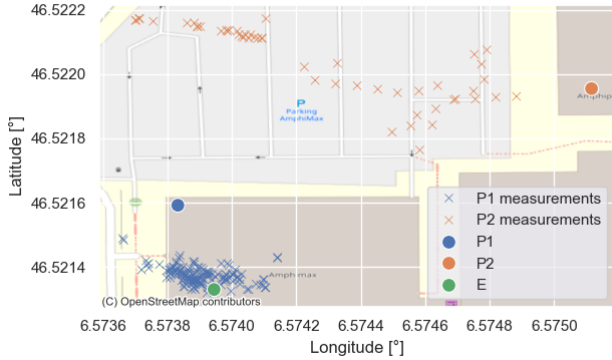
Figure 1: A geographical visualization of the UNIL dataset from [5]. E is the single localization that was recovered, while P1 and P2 are two proposed locations. Only deduplicated reference measurements for both proposals are shown. Note how reference measurements are not even on the same building as the proposal they were measured from.
