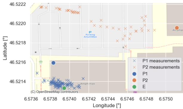
Figure 1: A geographical visualization of the UNIL dataset from [5]. E is the single localization that was recovered, while P1 and P2 are two proposed locations. Only deduplicated reference measurements for both proposals are shown. Note how reference measurements are not even on the same building as the proposal they were measured from.
